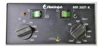
The stirring speed is adjusted with the right control knob. The temperature can roughly be adjusted with the left controller.
