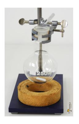
Stirring bars are used to continuously mix the reaction solution in a flask (see picture) or the heating bath.
