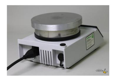
If the stirring hot plate is used without a contact thermometer, the the temperature connector (left) must be covered with the cap, as otherwise the heating function does not work.
