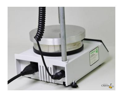
The contact thermometer is connected at the back of the stirring hot plate as shown in the picture.
