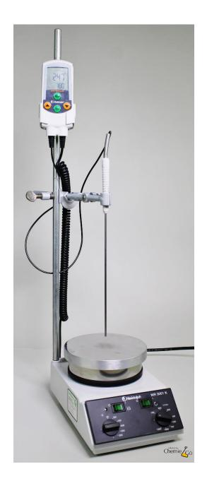
To accurately adjust the temperature of the heating bath, a contact thermometer is connected.
